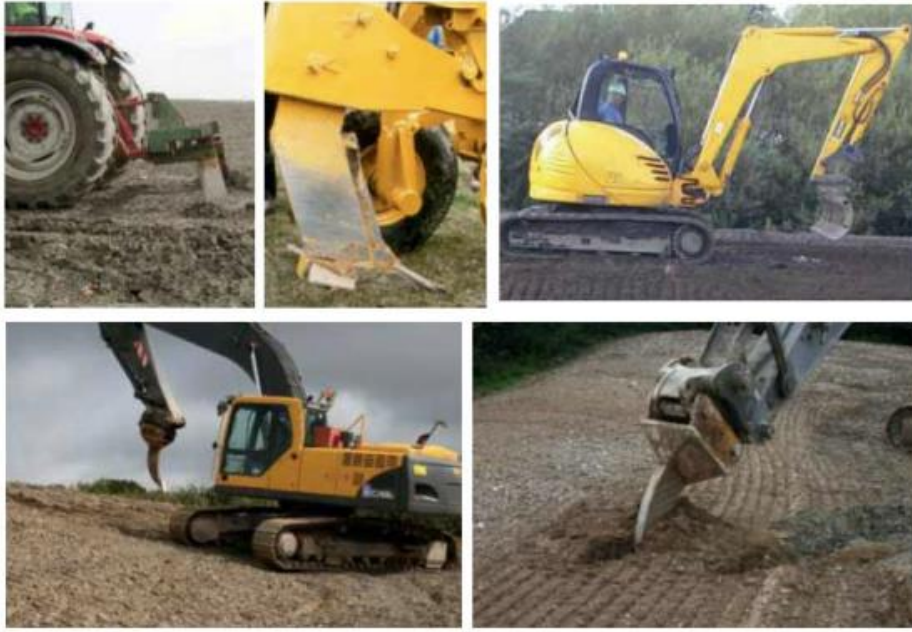
Figure 3-4: Top: (left to right) Tractor-drawn tines; Large winged ripping tine; Topsoil rake on 3-tonne excavator. Bottom: Single ripper tooth relieving compaction to a depth of 600mm
